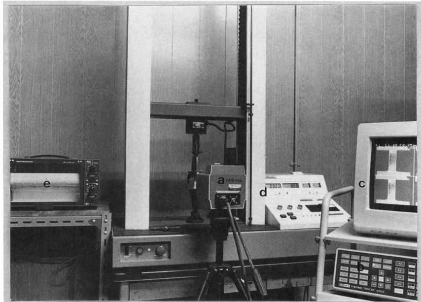
Figure 1 Setup of thermography for measuring surface temperature of the paper specimen under strain; (a) infrared camera; (b) control unit; (c) monitor display; (d) Instron-type machine; (e) recorder; (f) paper specimen.
